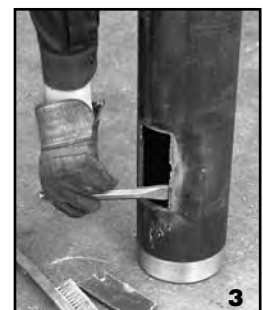
Remove slag and burrs.
