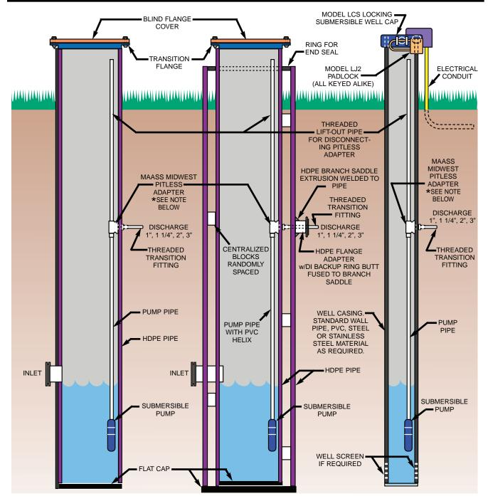
\*The following Maass Midwest Pitless Adapter models can be used: Model 304 JD-SS, Electroless Nickel Plated Models LDS, J or JC - N series (all with Viton O-Rings).
